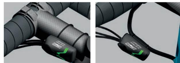
The special design of the interface lets the user choose between two different installation solutions: on the brake cable or on the handlebar mount.
