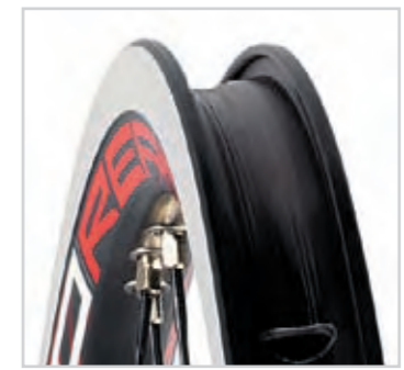
OVERSIZE UPPER BRIDGE: facilitates tire mounting.
