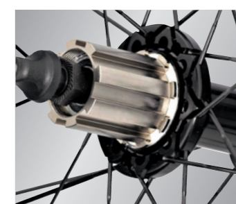
OVERSIZE FLANGE: enables efficient transmission of power to the wheel - increases torsional stiffness and the overall reactivity of the wheel.
