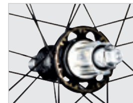
Rear hub in structural carbon with oversize flange
