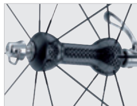
Front hub in structural carbon with variable thickness
