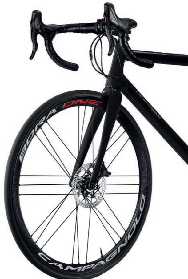
One piece solid construction to compensate for asymmetric forces from disc brakes
