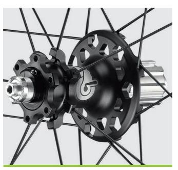
A truly efficient wheel is not only aerodynamically efficient but also must roll as smoothly as possible. CULT<sup>™</sup> technology employs ceramic bearings that are technologically superior to any competitors as well as Cronitect<sup>®</sup> steel, guarantees that your Campagnolo<sup>®</sup> are the highest performance solution you can find. Cronitect<sup>®</sup> steel is highly resistant to corrosion to the point that grease is unnecessary and only a small amount of oil is used.
