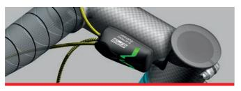
The analog signal received from the Ergopower™ control is transformed into a digital signal which is then sent to the Power Unit. The digital signal allows unique, error-free encoding of the signal transmitted by the Ergopower<sup>™</sup> units.
