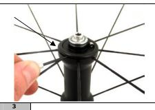
With a flat-bladed screwdriver remove the second protective cover. Make sure you do not damage the cover's locking teeth which would affect reassembling at a later stage.
