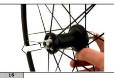
Insert the axle inside the body of the hub on the ratchet ring side.
