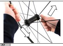
Insert the two 5mm hex wrenches inside the hexagons of the hub's body and tighten firmly. The right wrench (on the opposite side of the adjustment ring nut) remains fixed, the left wrench rotates clockwise.
