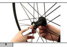
Push the axle inside the body of the hub until it reaches the other side.
