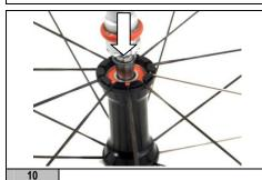
Check the stripping teeth are positioned correctly inside the bearing.
