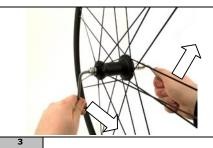
Insert the two hex wrenches inside the hex-drive of the Of the axle and end cap then firmly unscrew. The right side (on the opposite side of the adjustment ring nut) remains fixed, the left side end cap rotates counterclockwise to loosen the end cap.
