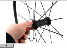
When the wheel has been in use it may be necessary to adjust the tolerance of the axle movement with respect to the bearings rolling in the cups and cones of the hub. To check whether the adjustment is necessary, hold the rim with one hand, in with the other move the axle to identify if the tolerance is too loose or tight.
