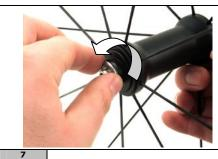
Loosen end cap (adjustment ring nut side).
