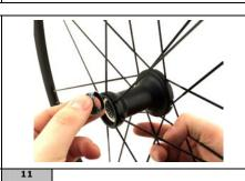
Remove the cone and the adjustment cone from the body of the hub.
