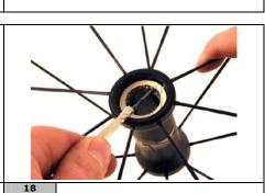
Remove the cone and the adjustment cone.
