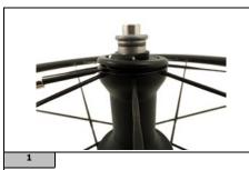
Remove the cover from the side of the adjustment ring nut with a small flat-bladed screwdriver.
