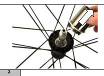
► To remove the freewheel body see OPERATION 004 (from 1 to 6)
