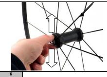
Check if the tolerance of the axle movement has been adjusted to satisfaction.
