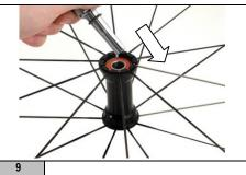
Insert the designated stripper on the internal diameter of the bearing.
