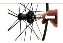
Check the cone is mates correctly into the bearing retaining ring.
