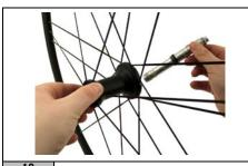
Remove the axle from the body of the hub.
