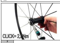
If the tolerance has been adjusted successfully, tighten the 2.5mm Allen screw with the torque wrench screwdriver set to 2.5 Nm (22 in.lbs). To reach the predefined torque, wait for the tool to indicate the proper torque.
