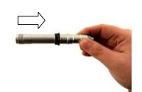
Insert the cone on the rear axle following the direction it should be inserted in. The larger diameter should face the axle.
