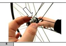
While removing the end cap, make sure you do not lose the spacer.
