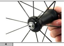
The indication that the adjustment ring nut will be loosened will be when the slot in the nut has a visible gap. Do not remove the screw from the adjustment ring nut
