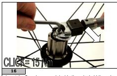
Insert the 5mm hex wrench inside the axle, hold the axle stationary and torque the lock nut with the a 17mm crows foot and a torque wrench.
