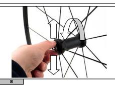
Check the movement of the axle when it rotates, if necessary repeat from point no. 2.
