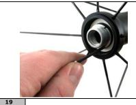
Manipulate it into position by using a small screwdriver. Push the adjustment cone in by pressing on various points of the circumference.
