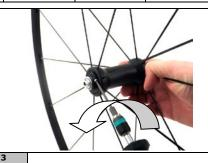
Once the screwdriver has been inserted inside the 2.5 screw, loosen the screw counter-clockwise 2 revolutions.
