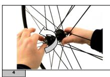
Loosen the axle end cap (adjustment ring nut side).
