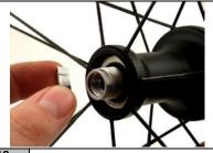
Insert the adjustment cone onto the axle mating into the cone from 17. The direction it should be inserted in. The larger diameter should face the outside of the hub's body.
