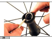
With a small screwdriver remove the bearing retaining ring making sure you do not damage it. Incorrect handling may cause the bearings to detach from the ring.
