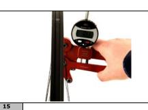
Check the tension of all the spokes of the wheel. If the tension value is low, repeat from point 7.
