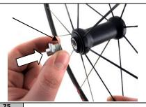
Inspect the axle end cap. If it is damaged, replace it. Insure that the small spacer is in place and install the end cap into the axle end.
