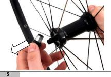
Loosen the threaded spacer by holding the left side of
