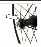
Insert the cover with the larger internal diameter on the body of the hub on the adjustment ring nut side. If it is damaged, replace it.
